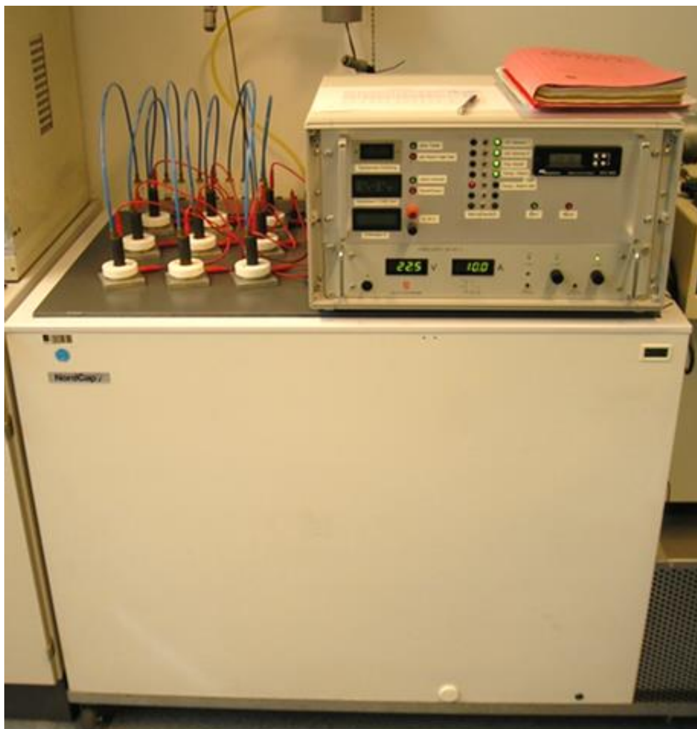
Fig. 3: Enrichment apparatus with nine electrolysis cells
