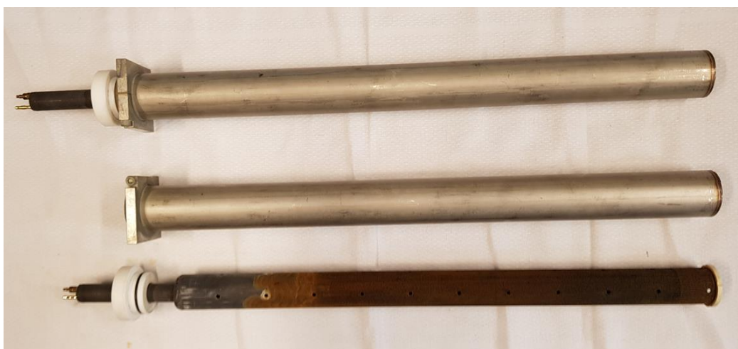
Fig. 4: Electrolysis cell (top) consisting of anode/outer part (center) and cathode/inner part (bottom)
