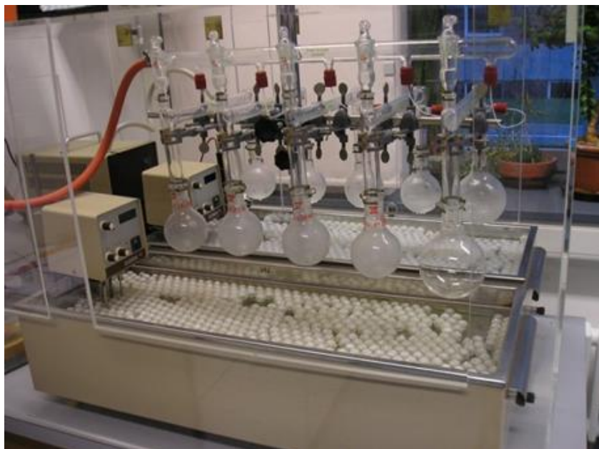
Fig. 1: Distillation apparatus with five distillation units
