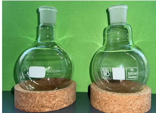
Fig. 3: Special design of a round-bottom flask (right) compared with a commercially available round bottom flask (left)
